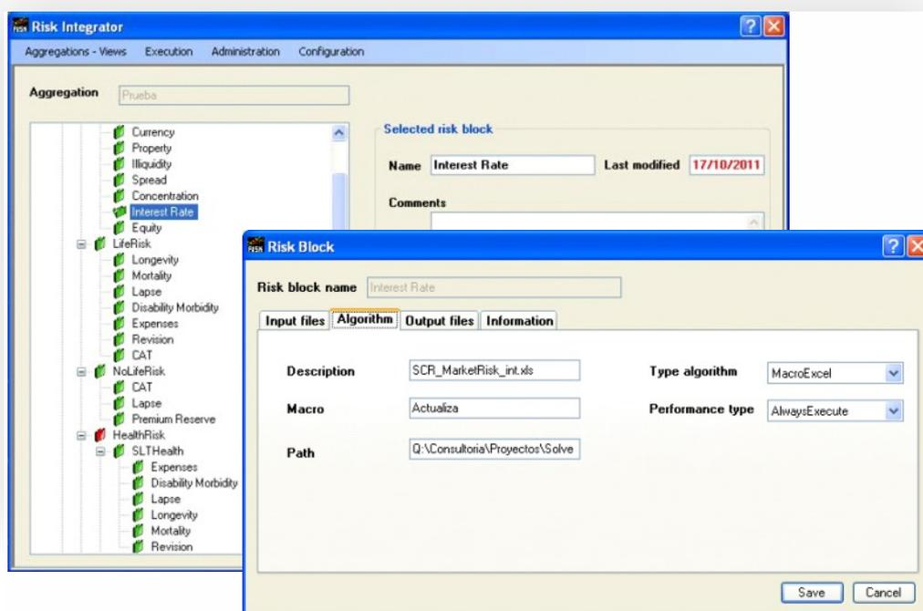
In a sequence of tabs on the Risk Block definition form, the user defines the input files, the algorithm (and its tool), the output files (both model results and reporting) and also information relating to the documentation of the work step (high-level comments plus references to detailed documentation).
